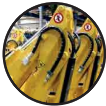
Auxiliary line for hydraulic tool applied to the arm supply
